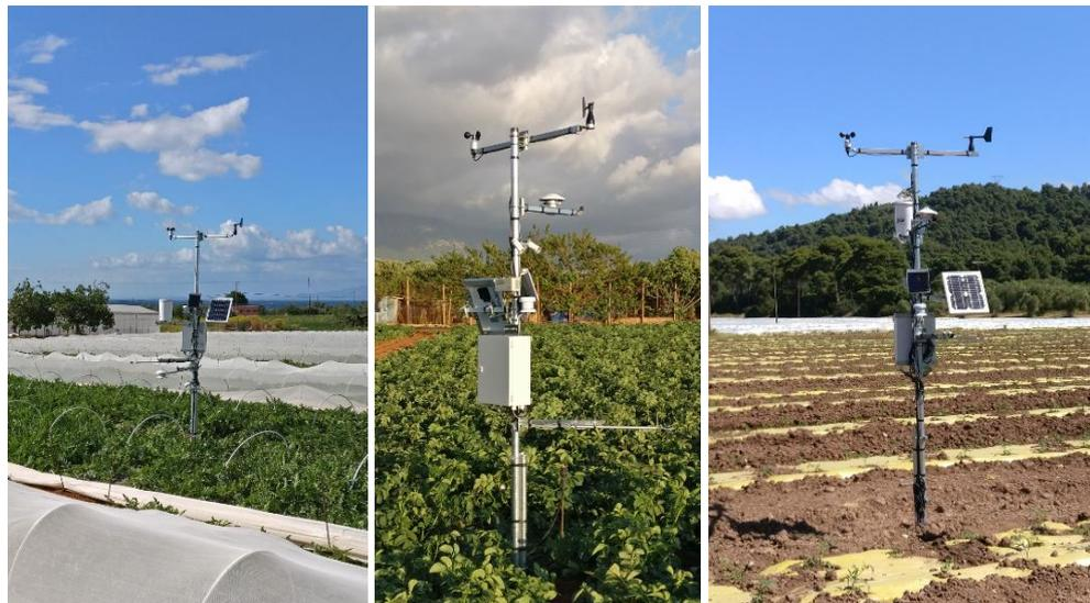
The stations are self-powered. The power supply is made via two complete independent photovoltaic systems. The first one supplies the telemetry system and the second one supplies the sensors. This technique was applied for the first time from SCIENTACT 15 years ago, providing excellent stability to systems with multiple sensors.
